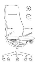
Control located on the left side under the seat.
